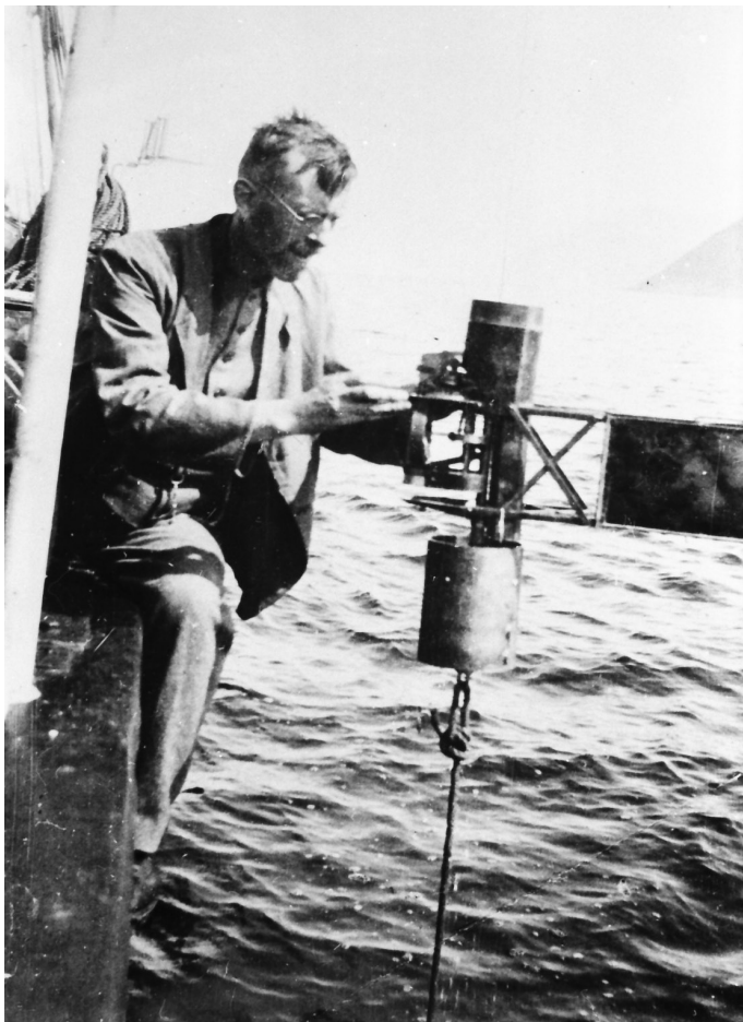
Ekman making current measurements using the current meter designed him. Source: Bergen University.
